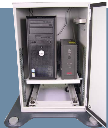
Below: Console features a locking cabinet which protects PC from tampering.
